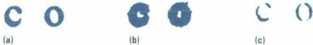
Fig. 3. The results of different threshold settings. (a) Normal setting. (b) Threshold set too low. (c) Threshold set too high.
